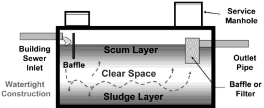
A septic tank looks like the illustration above. The size of the tank depends upon the number of bedrooms in the house, not the number of people or plumbing fixtures. The sizes range from 750 gallons on up and may be configured as one or two septic tanks. Having two septic tanks (or a two compartment septic tank) increases detention time of the waste water, which helps to further reduce the suspended solids that could flow into the drainfield.
