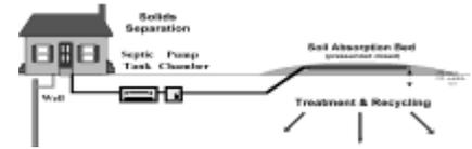
This system is similar to the At-Grade with washed sand placed on the plowed surface and the drainfield bed constructed in the sand. When finished, this will be approximately 3-4 ft above the grade
