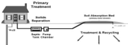
This system is built on top of the original grade, area is plowed, stone is placed on top of the plowed surface along with the distribution pipes. System is covered with soil and is approximately 2 ft above the grade.
