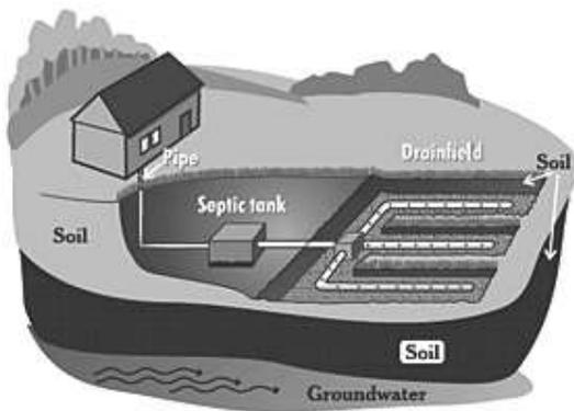
A septic tank is typically the first component of a septic system. A system can be as simple as a septic tank with an efficient filter screen and drainfield or include any number of add-ons, such as an aeration tank, sand filter, pump/siphon chamber or sand mound.
